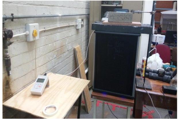
**Figure 5.** Setup for Thermal Conductivity
