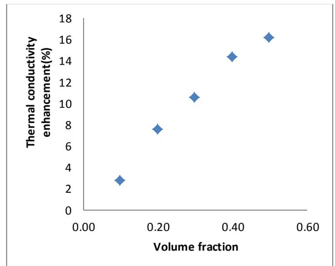
**Figure 7.** Thermal conductivity enhancement For Palm Kernel Fibre nanofluid with water and Ethylene Glycol(50:50) Base Fluid.
