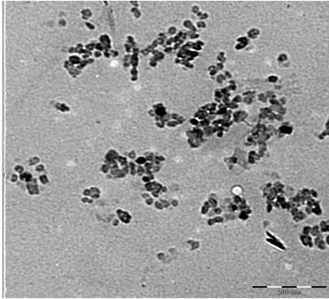
**Figure 4.** TEM Image of Palm Kernel Nanoparticles
