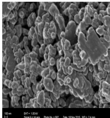
**Figure 3.** SEM Image of Palm kernel Fibre Nanoparticles
